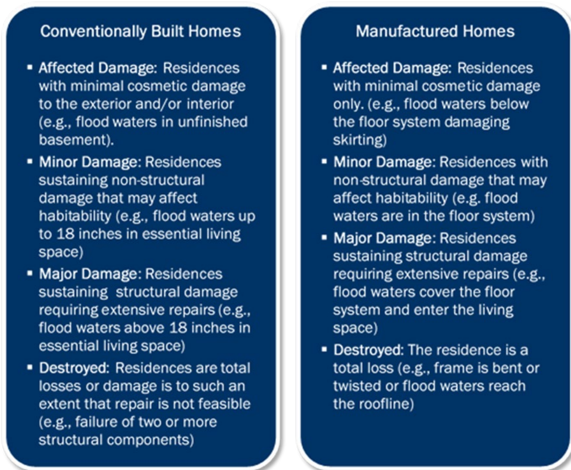
Figure 3: Damage Levels and Criteria for Homes
